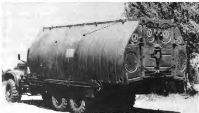
Figure 6-50. PMP heavy folding bridge. This new-type "ribbon bridge" provides a rapid-assembly heavy (class 60) bridge. The sections are carried folded on the backs of trucks. The trucks back up to the water's edge and dump their spans which open automatically as they hit the water. The bridge is assembled in the water along the shoreline and positioned by power boats.
